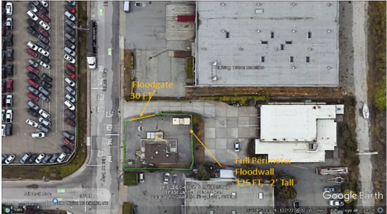
Figure 13-Pump Station No.4 with Proposed Floodwall/Retaining wall
